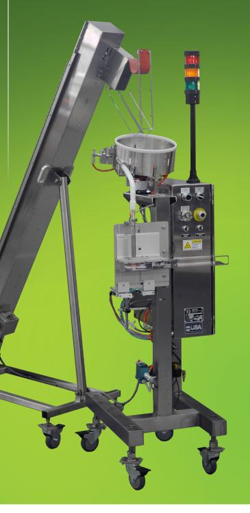
Low Cost and Highly Reliable Automatic <u>Canister Inserter</u>
